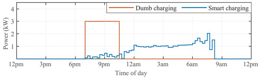
**Figure 1.** Comparison of charging-power profile of an EV.
