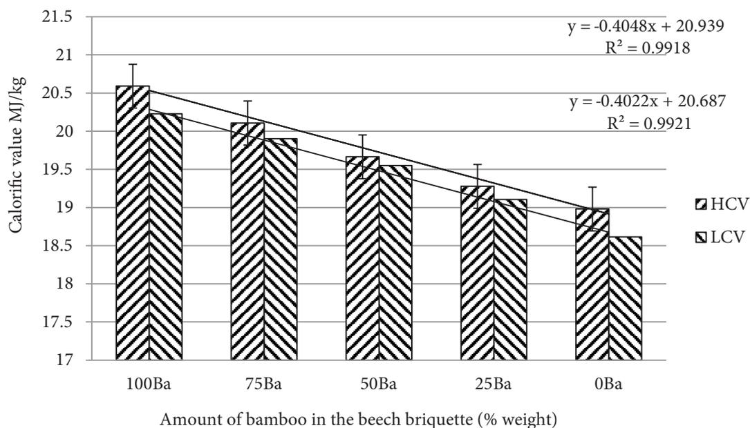
**Figure 6.** Higher calorific value (HCV) and lower calorific value (LCV) of briquettes with different fractions of bamboo wood.
