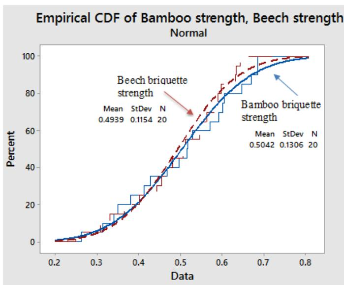
Figure 12. Empirical cumulative distribution function (CDF) of the breaking strength of bamboo and beech briquettes.
