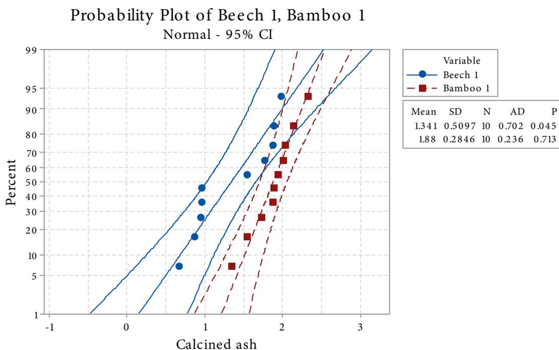
Figure 8. Calcined ash content of beech and bamboo biomasses.
