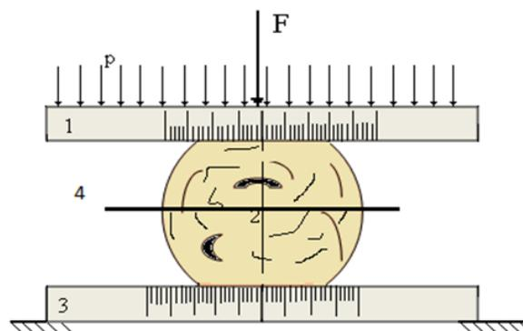
**Figure 2.** Superior platen. 2: Briquette. 3: Inferior platen. 4: Breaking section. P: Specific pressure. F: Force (Spîrchez and Lunguleasa, 2016).
