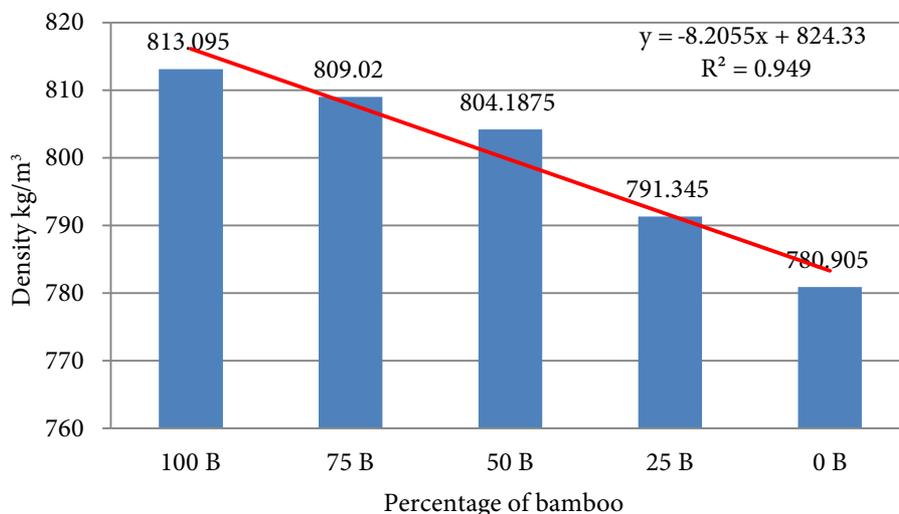
Figure 4. Density of briquettes with different bamboo wood fractions (B).
