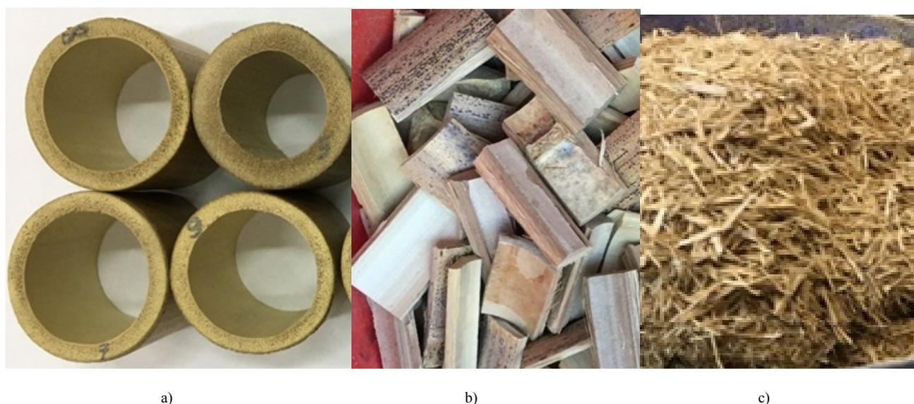
**Figure 1.** Bamboo wood. a) 40 mm long samples, b) shreds, c) particles (chips).
