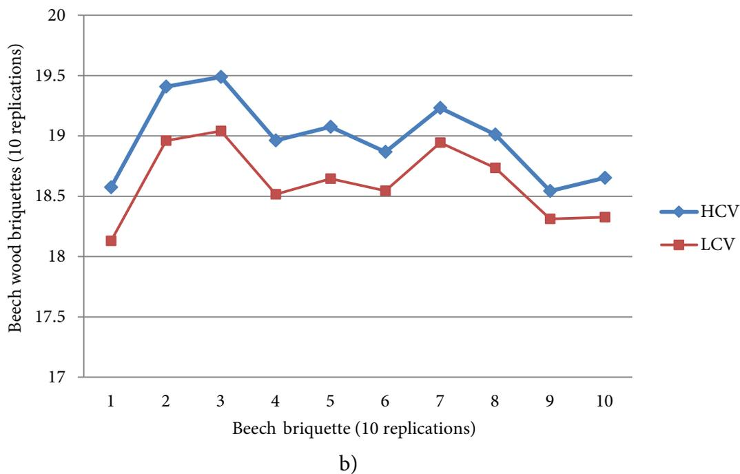
**Figure 5.** Higher (HCV) and lower (LCV) heating (calorific) values of briquettes a) Bamboo wood briquettes, b) beech wood briquettes.
