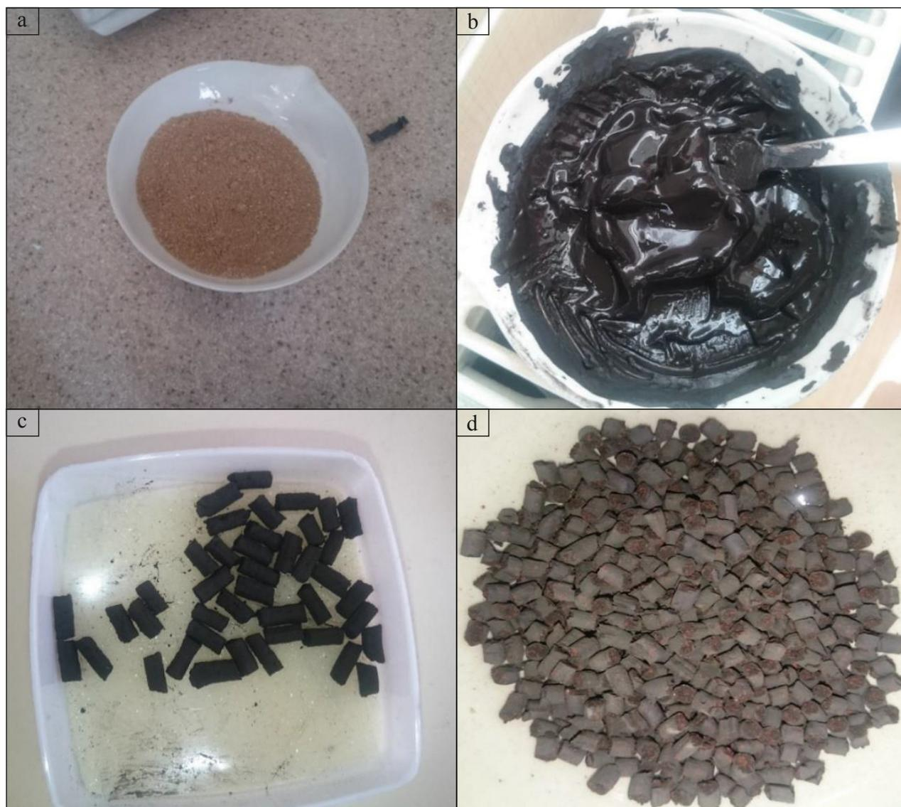
**Figure 3.** The production stages of adsorbent, (a): Li-Mn mixture are prepared by 1/1 molar ratio, (b): pasty mixture, (c): sized and dried mixture and (d): the heated mixture at 650 °C.
