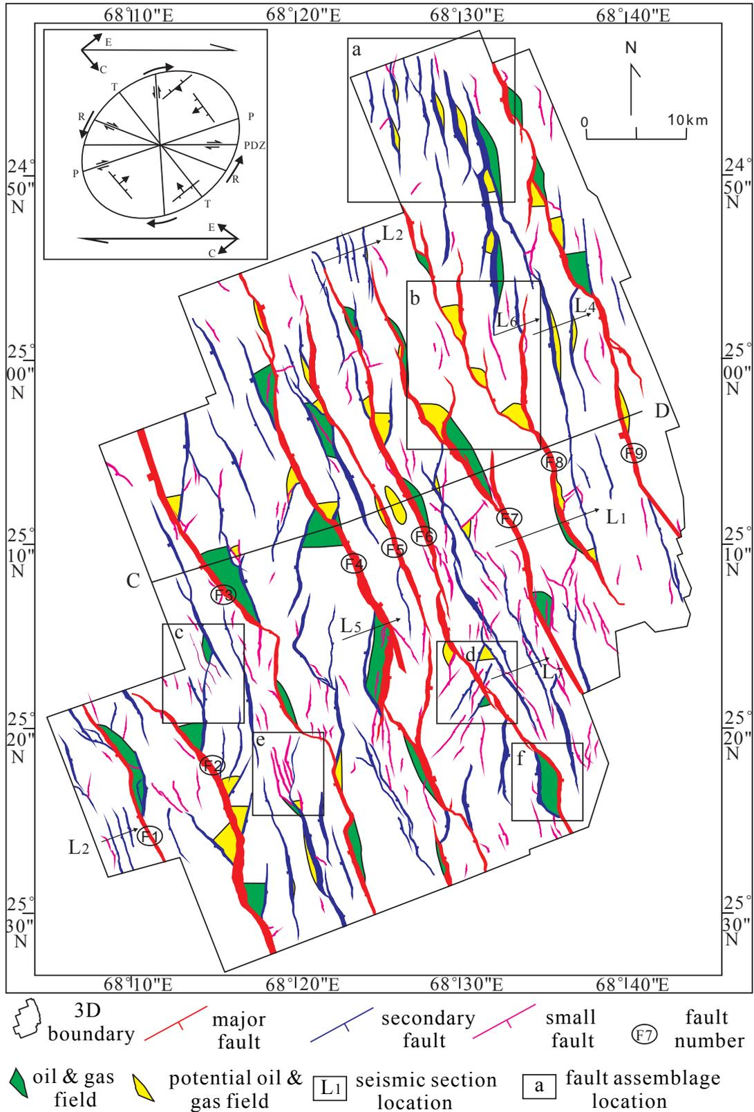
**Figure 3.** Fault system and discovered oil field map of the Lower Cretaceous. Note: The picture on the top left is a dextral slip shear model map. PDZ: the priority displacement zone, E: extended component, C: compressional component, T: tensional fracture, P: synclastic shear fracture, R: riedel shear fracture.
