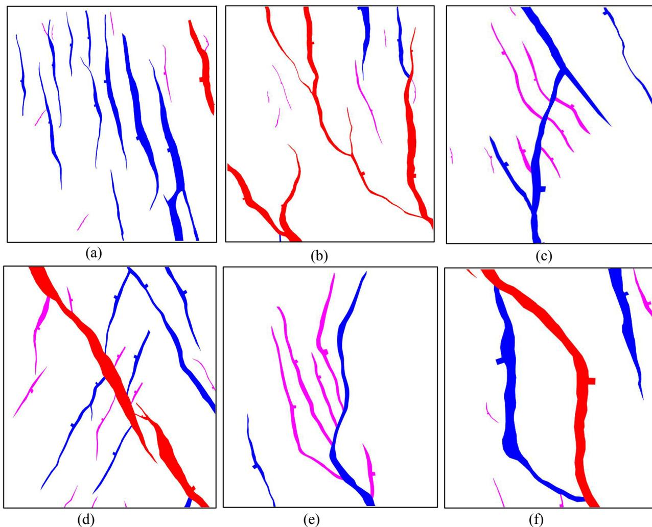
**Figure 5.** Typical plane assemblage patterns of transtensional faults. The fault location is shown in Figure 3). (a) En echelon pattern; (b) broom pattern; (c) pinniform pattern; (d) comb pattern; (e) horsetail pattern; (f) diamond pattern.
