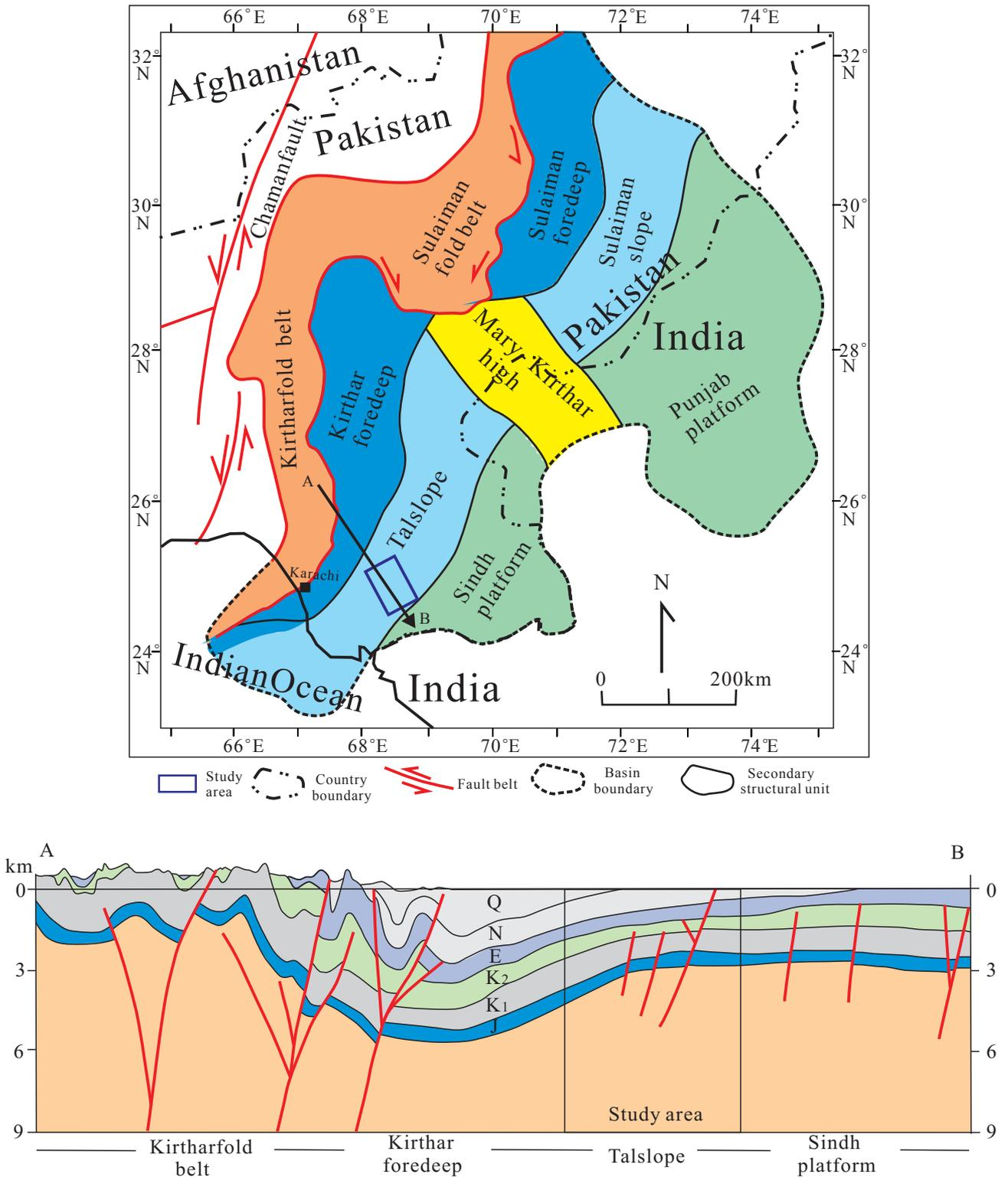
**Figure 1.** Structural elements of Indus Basin and location of the study area (a) and regional stratigraphic framework from northwest to southeast (b) (modified from Zuxi et al., 2005).
