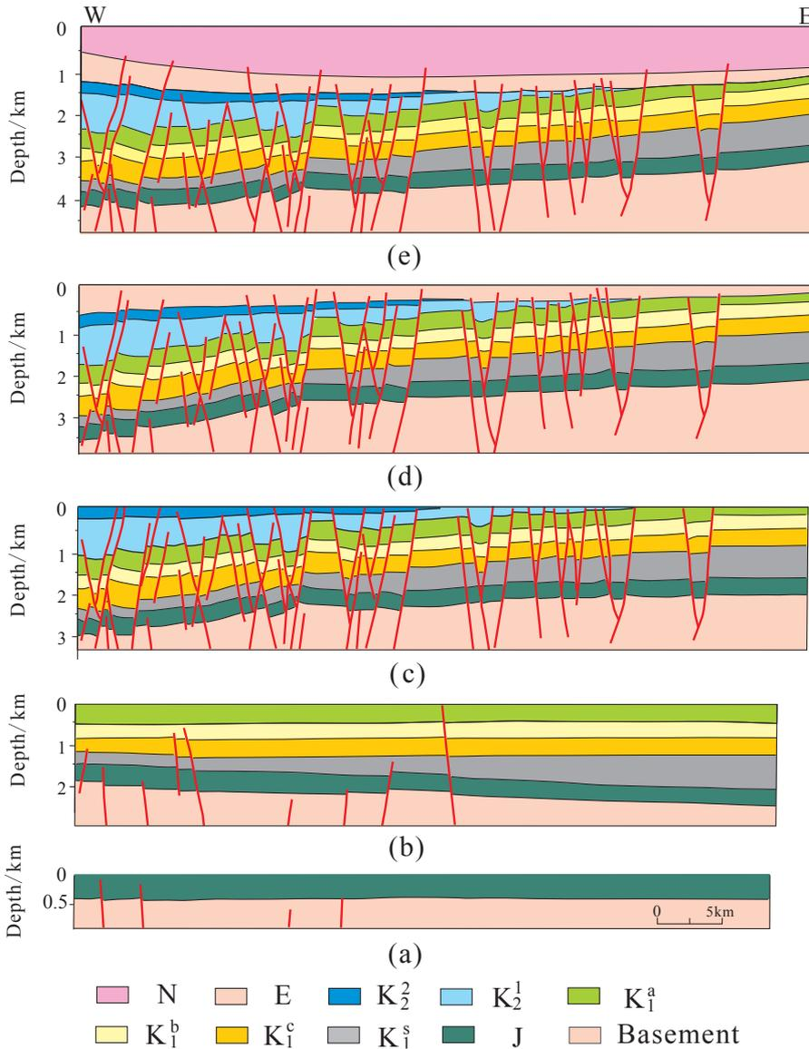
**Figure 8.** W-E seismic profile of fault structure evolution from Jurassic to present. (a) Rifting in Jurassic; (b) passive continental margin stage in Early Cretaceous; (c) diagonal extension stage in Late Cretaceous; (d) thermal subsidence stage in Paleocene; (e) plate collision and tectonic reverse since Eocene.
