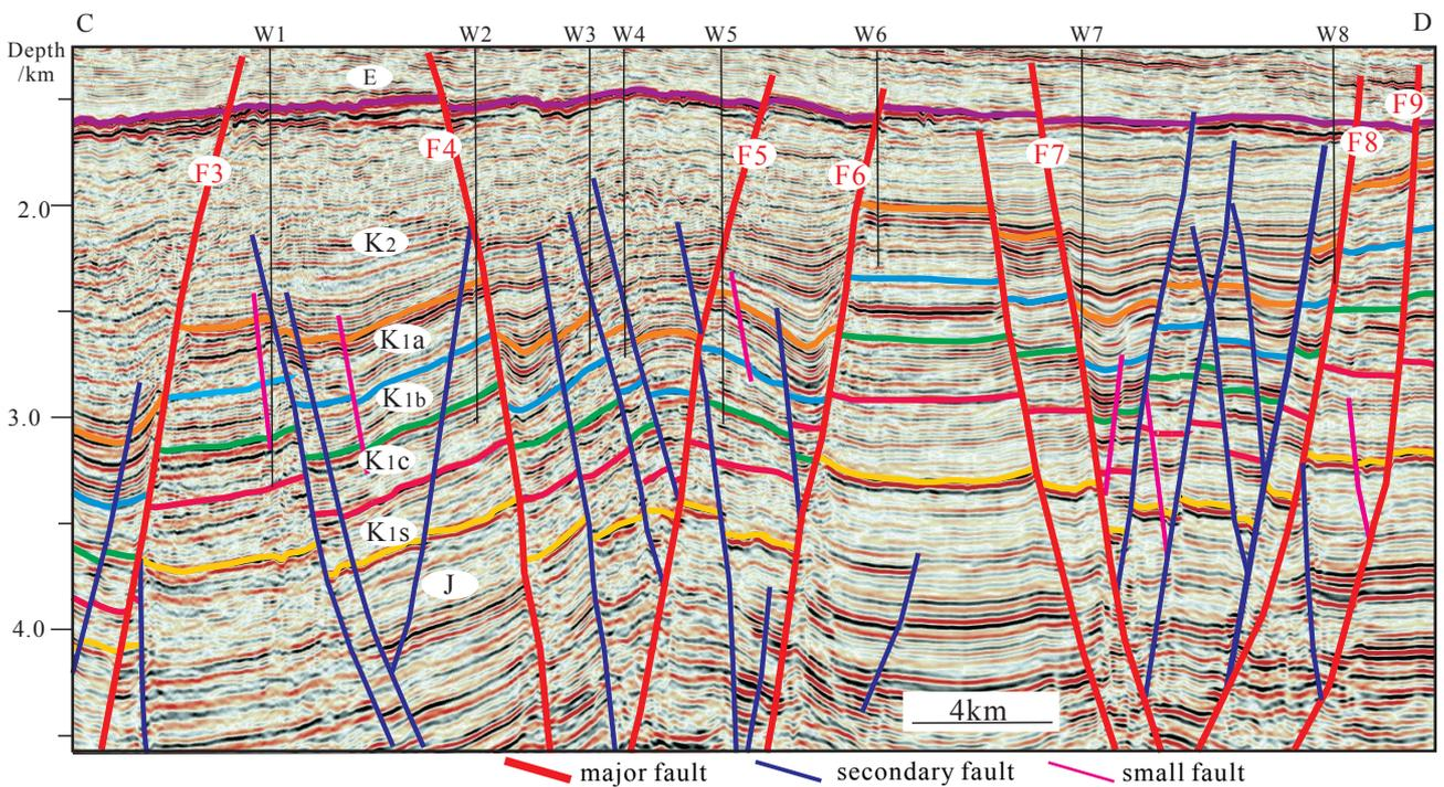
**Figure 4.** Seismic interpretation section showing the transtensional fault structure (The section location is shown in figure 3 “line CD”).
