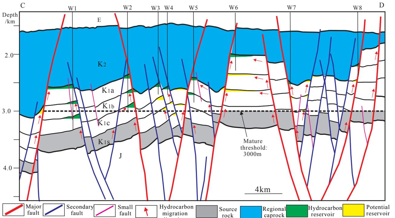
Figure 12. Hydrocarbon migration and accumulation model (The section location is shown in figure 3 “line CD”).
