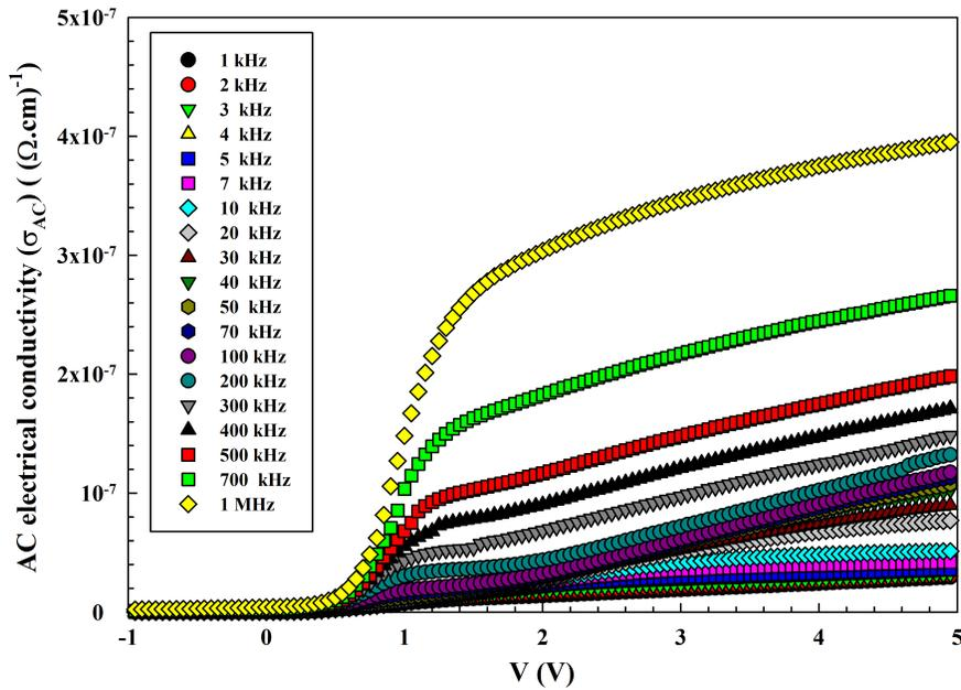
Figure 8.  $\sigma_{AC}$ - $V$  plot for Al/Mg<sub>2</sub>Si/p-Si SD in a wide frequency range.
