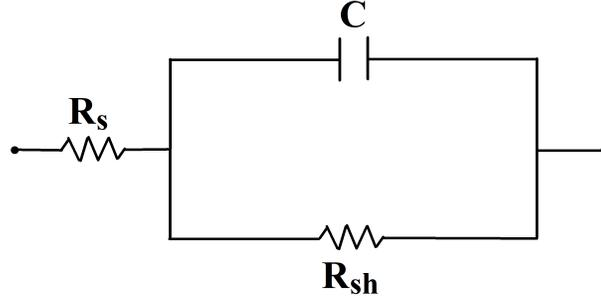
**Figure 2.** The equivalent electrical circuit for Al/Mg<sub>2</sub>Si/p-Si SD.
