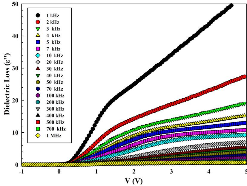
Figure 4.  $\epsilon'' / V$  plot for Al/Mg<sub>2</sub>Si/p-Si SD in a wide frequency range.
