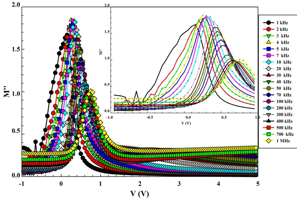
Figure 7.  $M''$ - $V$  plot for Al/Mg<sub>2</sub>Si/p-Si SD in a wide frequency range.
