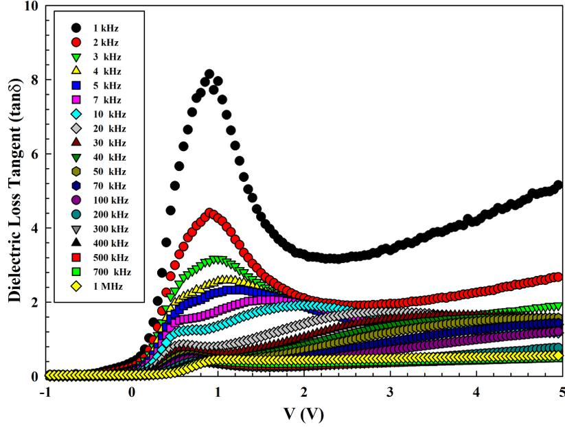
**Figure 5.**  $\tan \delta$ -V plot for Al/Mg<sub>2</sub>Si/p-Si SD in a wide frequency range.
