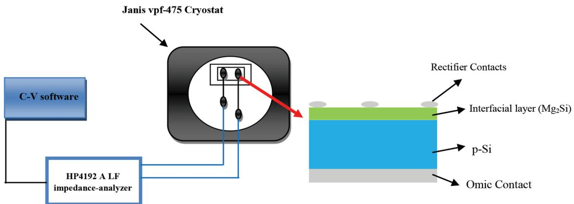
**Figure 1.** The capacitance and conductance measuring system and the cross section of Al/ $\text{Mg}_2\text{Si}$ /p-Si SD.
