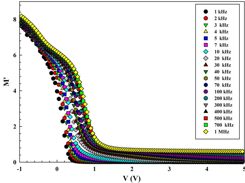
**Figure 6.**  $M'$ - $V$  plot for Al/ $Mg_2Si$ /p-Si SD in a wide frequency range.
