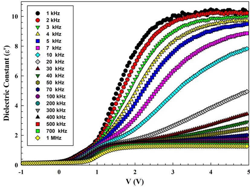
Figure 3.  $\epsilon' / V$  plot for Al/Mg<sub>2</sub>Si/p-Si SD in a wide frequency range.
