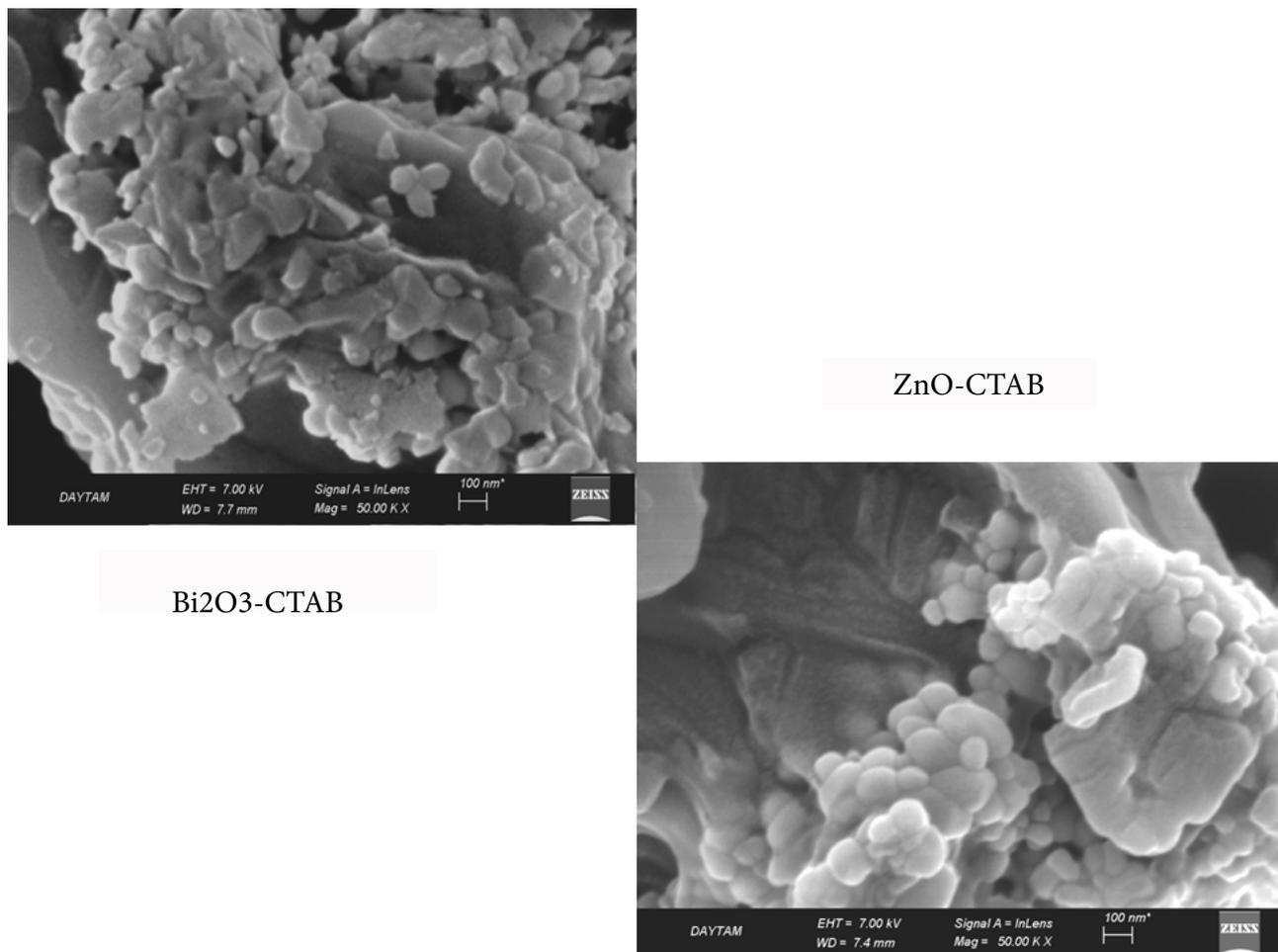
**Figure 8.** SEM images of  $\text{Bi}_2\text{O}_3$ -CTAB and ZnO-CTAB catalysts.
