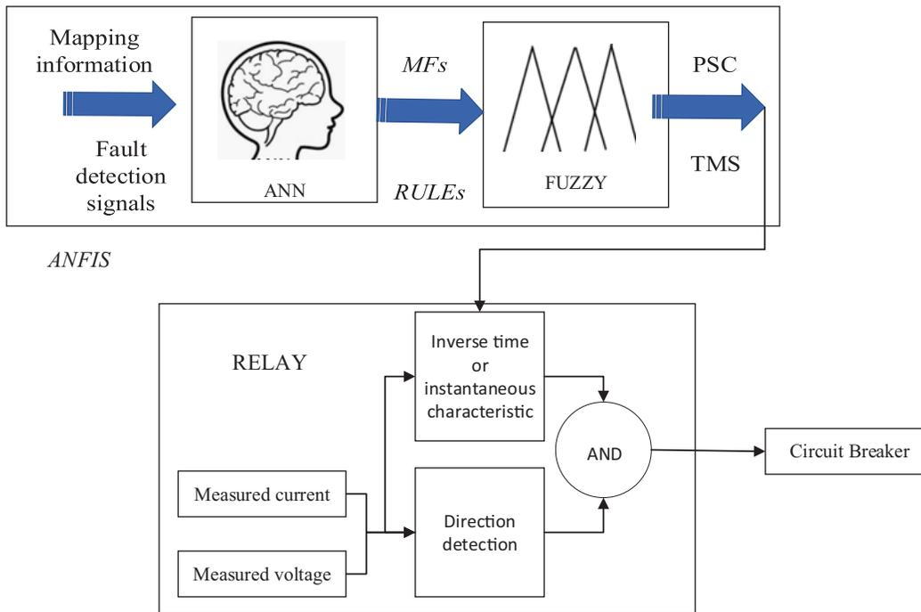
Figure 4. Flow diagram of adaptive relaying scheme using ANFIS.
