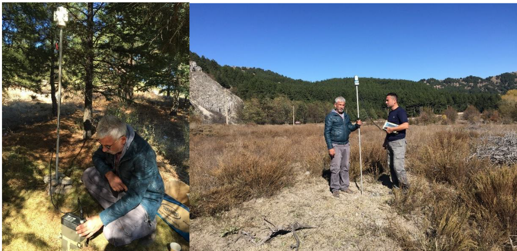
Figure 4. Pictures from the magnetic survey. Base station on the left and mobile measurement station on the right.
