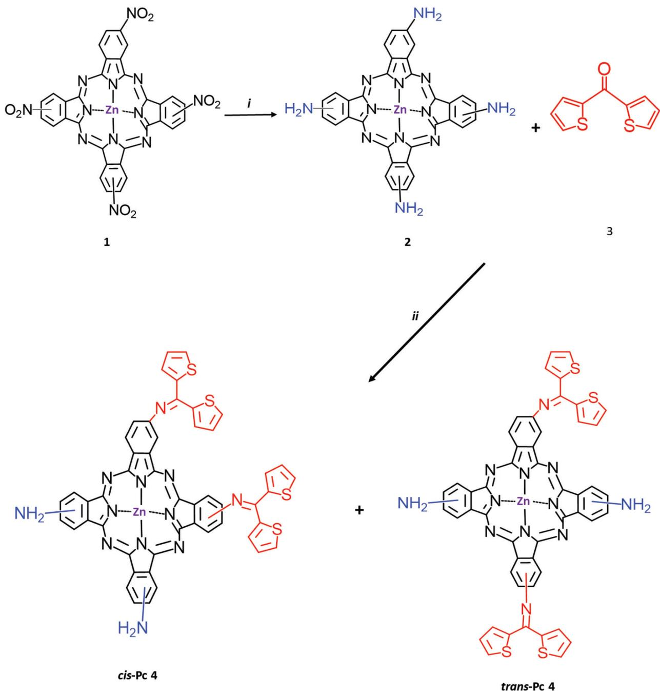
**Figure 1.** Synthetic route of Pc 4: (i) Pd/C, hydrazine hydrate, 1,4-dioxane; (ii) dry DME, *p*-TsOH·H<sub>2</sub>O, 48 h, reflux.
