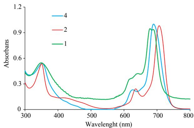
**Figure 2.** UV-Vis absorption spectra of complex **1**, **2** and **4** in THF ( $1.0 \times 10^{-5}$  M).
