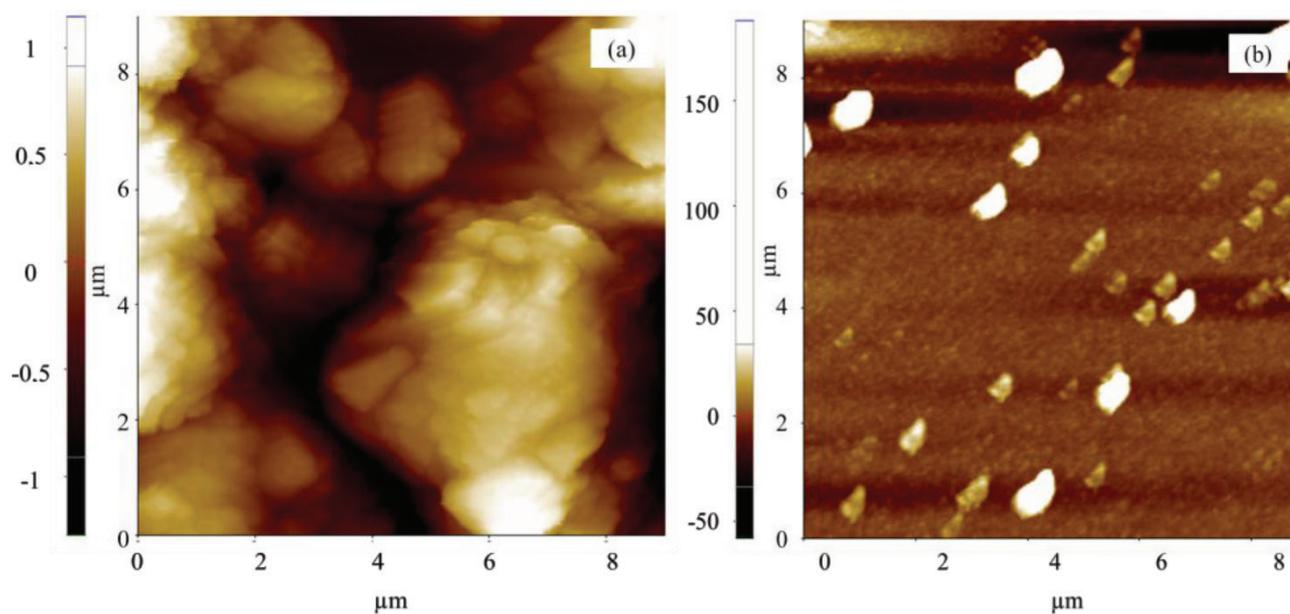
**Figure 3.** AFM topography of the films with 4.0:1.0 (a) and 2.5:1.0 (b) blend ratios.
