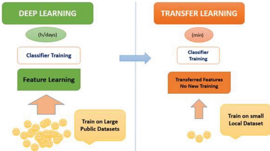
Figure 2. Comparison of building a network from scratch (left) and by transfer learning (right).
