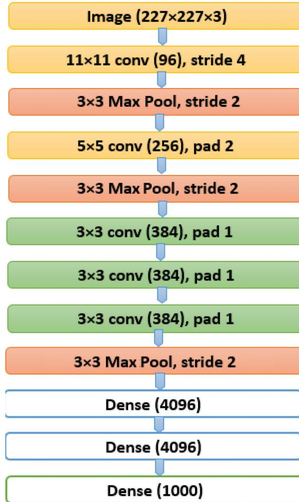
Figure 4. AlexNet architecture.
