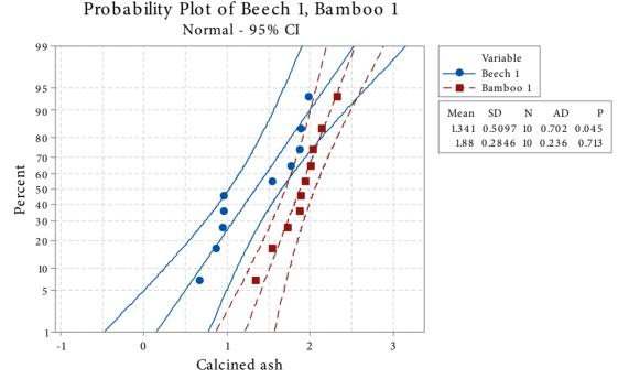
Figure 8. Calcined ash content of beech and bamboo biomasses.
