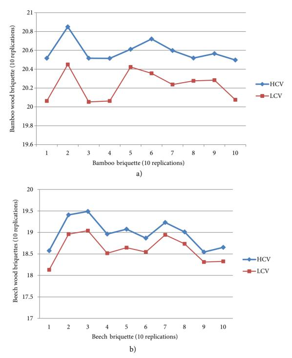
Figure 5. Higher (HCV) and lower (LCV) heating (calorific) values of briquettes a) Bamboo wood briquettes, b) beech wood briquettes.
