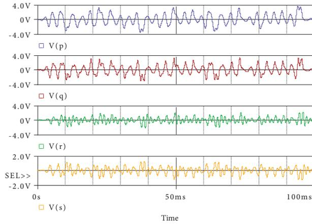
Figure 7. The outputs of the system (9) state variables ( $p, q, r, s$ ) of the analog electronic circuit design using CCII+s.
