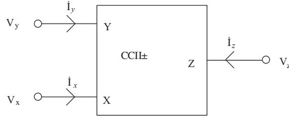
Figure 5. General structure of a CCII± device.
