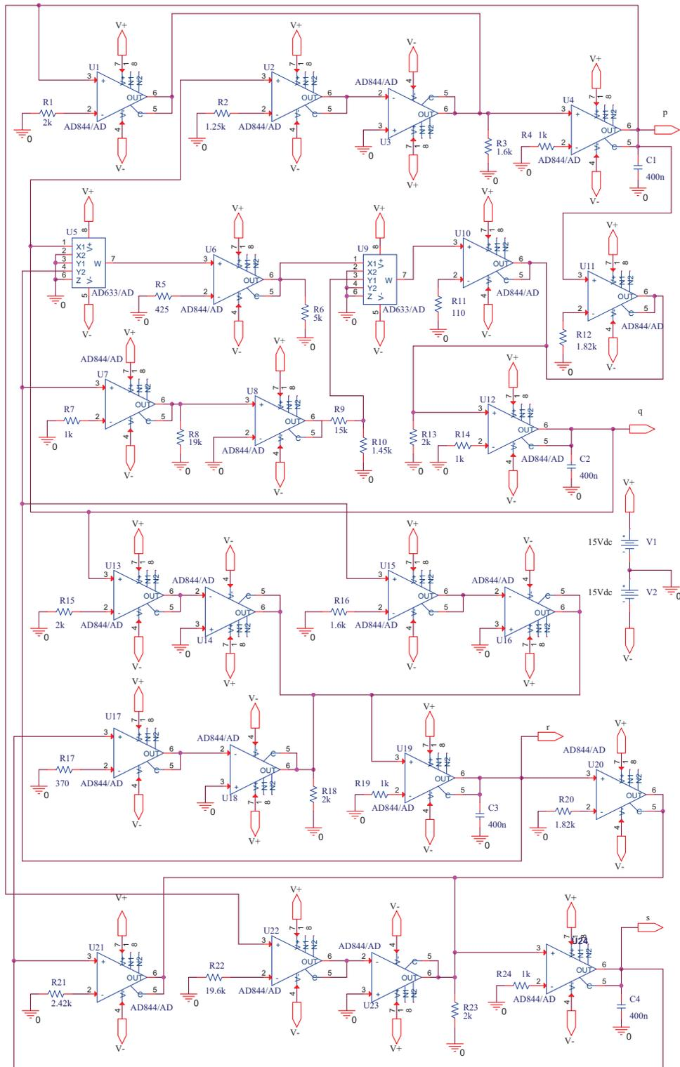
Figure 6. The electronic circuit design using CCII+s of the introduced NHS (9) for real engineering applications.
