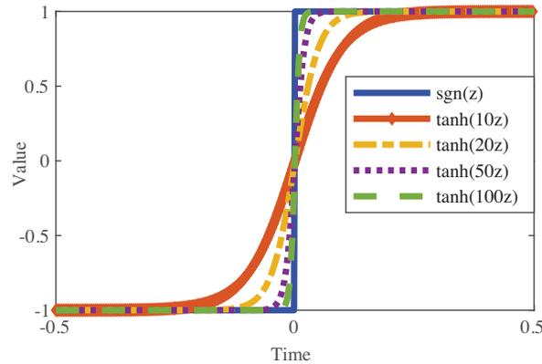
**Figure 1.** The comparison graph showing that the signum function and the hyperbolic tangent function can be used interchangeably.
