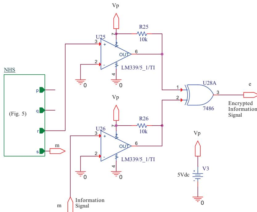
**Figure 9.** The analog electronic circuit of the designed encryption application using the introduced NHS.
