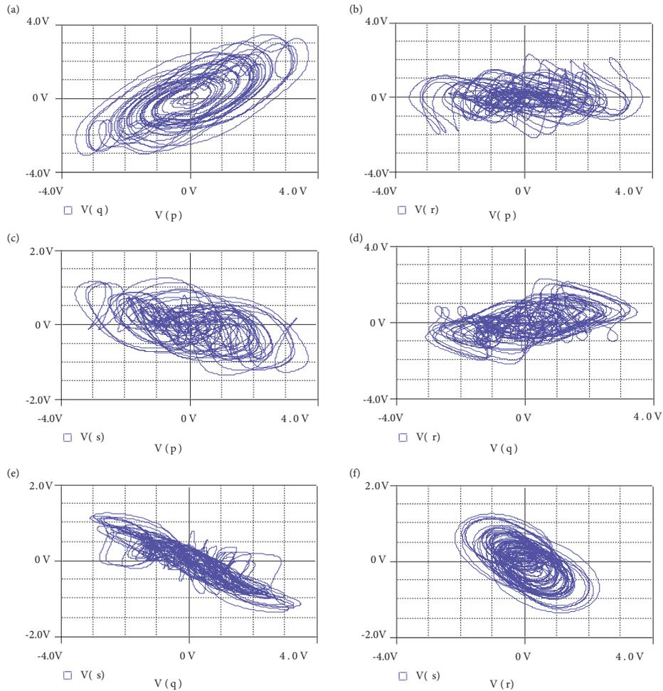
Figure 8. The phase characterization of the analog electronic circuit design using CCII+s of system (9) (a) for  $p - q$  state variables, (b) for  $p - r$  state variables, (c) for  $p - s$  state variables, (d) for  $q - r$  state variables, (e) for  $q - s$  state variables, (f) for  $r - s$  state variables.
