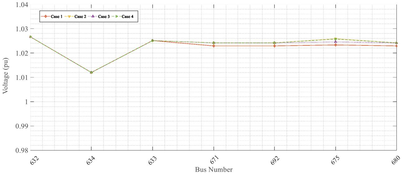
**Figure 11.** Voltage magnitudes of three-phase buses under cases consisting of different DG integration schemes and loading factors at 12.00 time interval.
