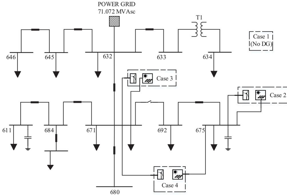
**Figure 4.** DG integrated 13-bus IEEE test system with variable loading conditions.
