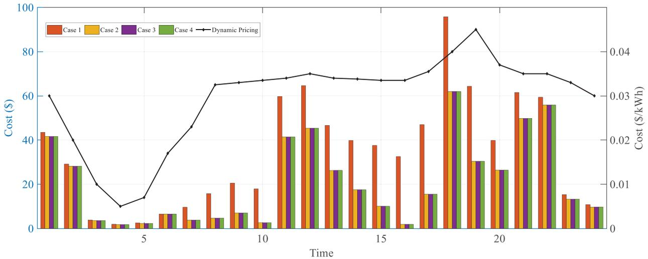
Figure 16. Daily costs of DG integrated test system for each case and dynamic pricing data.
