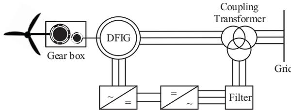
**Figure 3.** Integration of the DFIG consisting of wind power with full converter interface [21].
