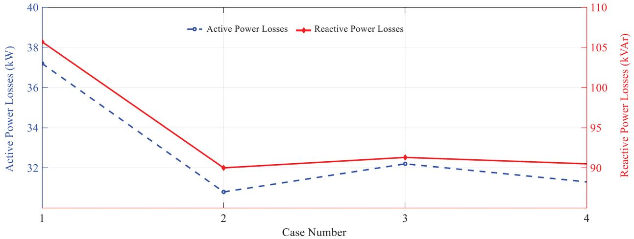
Figure 15. Active and reactive power losses of entire 13-bus test system under different cases and full loading condition.
