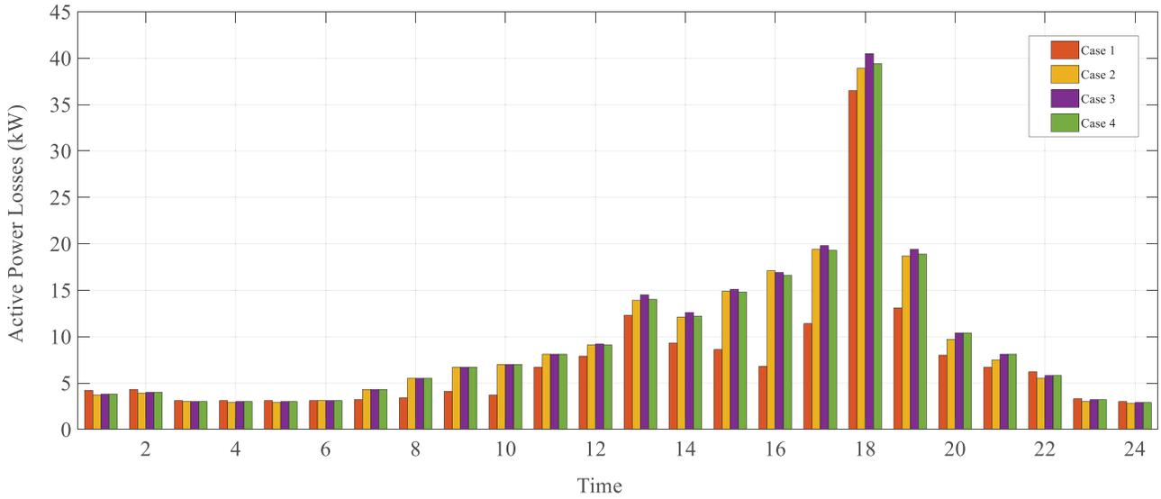
**Figure 13.** Active power losses of the entire 13-bus test system under cases consisting of different DG integration schemes and loading factors.
