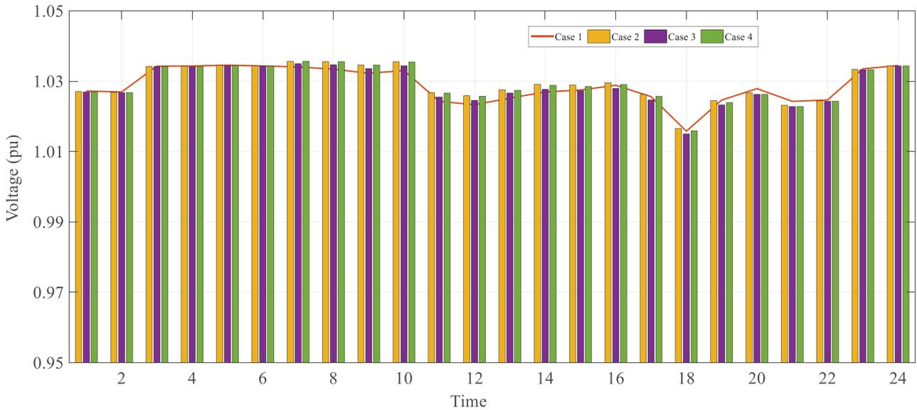
**Figure 8.** Voltage magnitude of bus 675 under cases consisting of different DG integration schemes and loading factors for a daily time scale.
