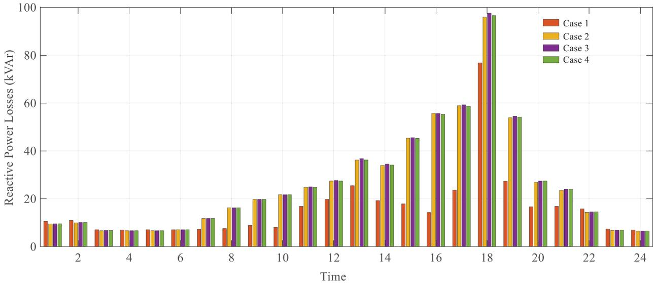
**Figure 14.** Reactive power losses of entire 13 bus test system under cases consisting different DG integration schemes and loading factors.
