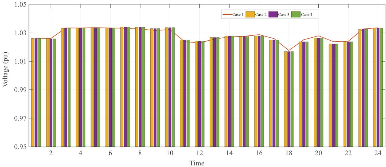
**Figure 7.** Voltage magnitude of bus 671 under cases consisting of different DG integration schemes and loading factors for a daily time scale.
