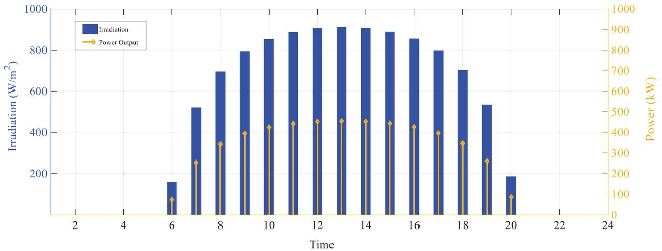
**Figure 10.** Daily variable solar irradiation (blue column) and power output of 500 kW PV system (yellow column) used for the simulation cases.
