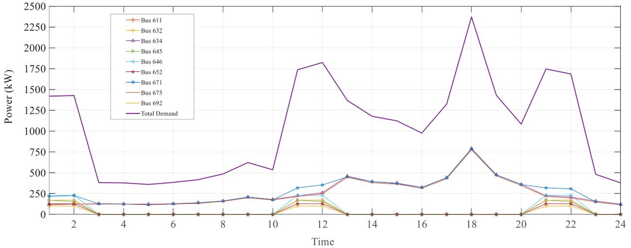
**Figure 5.** Power demand profile of each three-phase bus and total system for a daily time scale.
