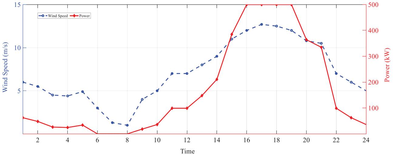
**Figure 9.** Daily variable wind speed (blue dotted line) and power output of 500 kW WTG (red line) used for the simulation cases.
