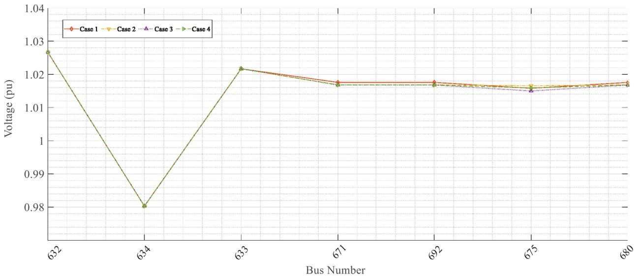
**Figure 12.** Voltage magnitudes of three-phase buses under cases consisting of different DG integration schemes and loading factors at 18.00 time interval.
