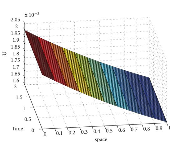
**Figure 1.** Exact :Surface of the wave for  $a = 1$ ,  $b = 1$ ,  $c = 0.001$ ,  $h = 0.1$ ,  $\Delta t = 0.005$ .
