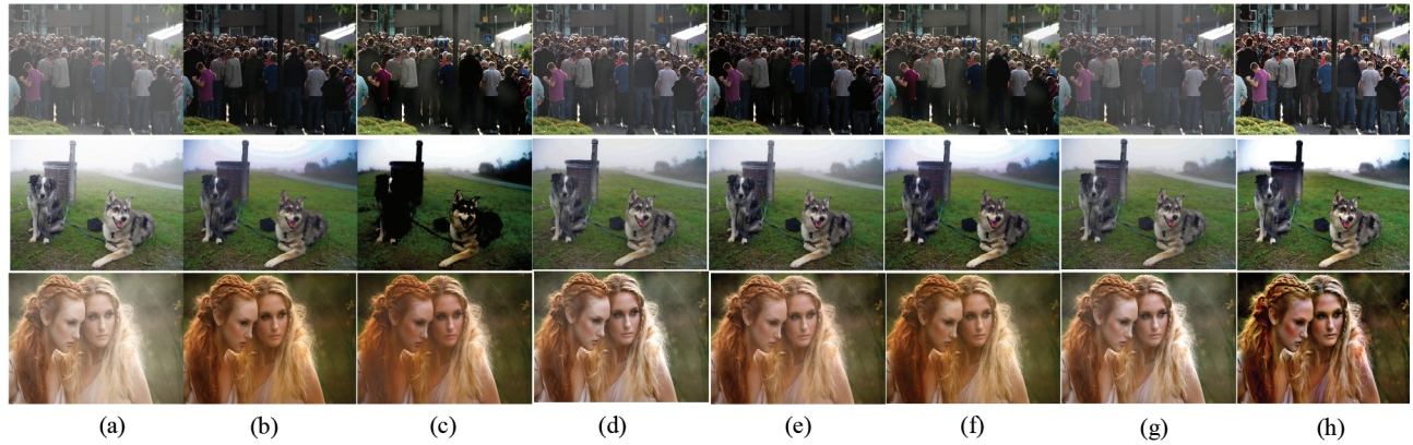
Figure 7. Visual comparison on challenging foggy images (a) foggy image (b–g) restored image using [3], [4], [12], [13], [15], [17], and (h) proposed method.
