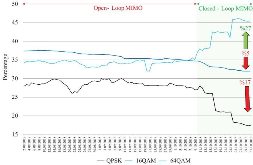
Figure 3. Modulation usability (%) KPI obtained from the real-time testbed.
