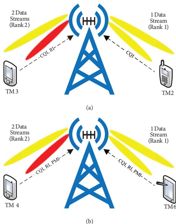
**Figure 1.** Operation of MIMO schemes with different classes of UEs (a) Open-loop MIMO, UEs reporting CQI and RI (b) Closed-Loop MIMO, UEs reporting CQI, RI and PMI.
