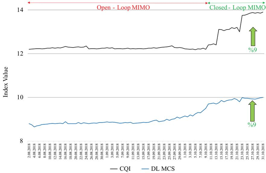
Figure 5. Average CQI and average downlink MCS KPI obtained from the real-time testbed.
