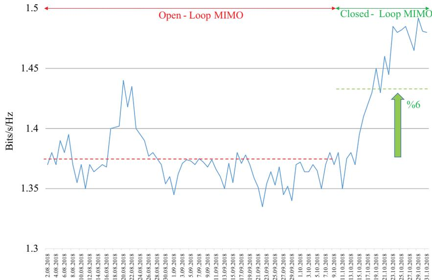
**Figure 2.** Comparison of downlink spectrum efficiency of open-loop and closed-loop MIMO.
