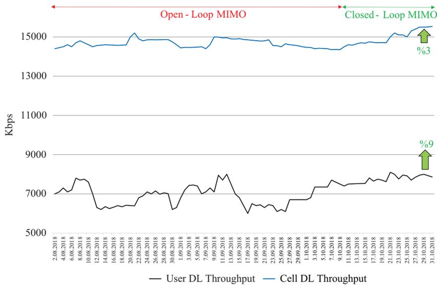
Figure 4. User and cell downlink throughput KPI obtained from the real-time testbed.
