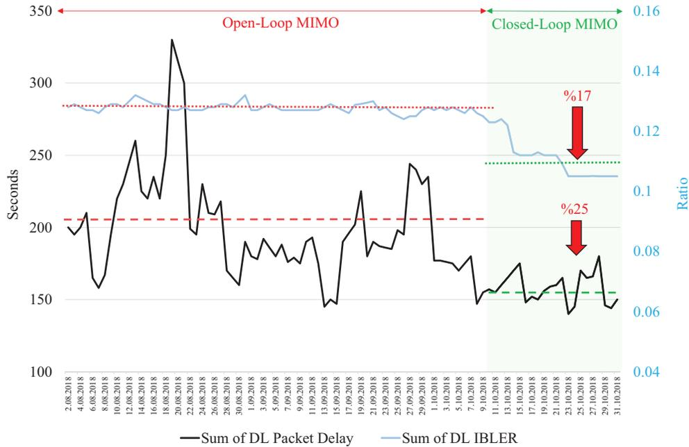
Figure 6. Comparison of sum of delay and IBLER between open-loop and closed-loop MIMO.
