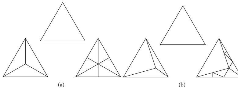
**Figure 1.** Two commonly applied subdivision technique for triangular shapes, (a) the division based on the center point, (b) division based on the projected point. The left division is the first iteration, the right is the redivision to obtain regular triangles.
