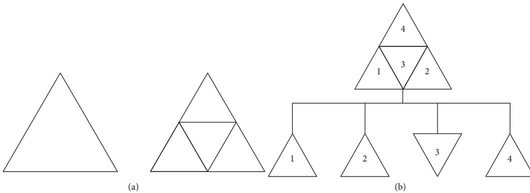
**Figure 3.** The subdivision of the triangular element (a) proposed subdivision technique applied to a triangular element, and (b) the parent and its four children in tree structure.
