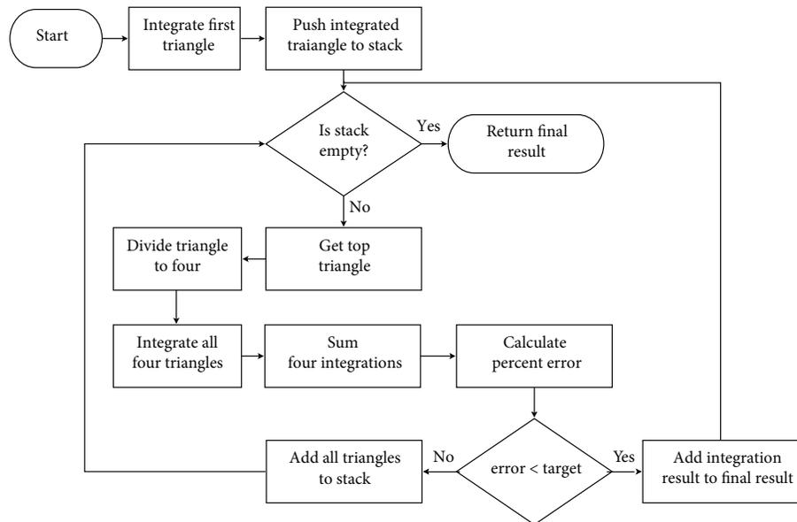
Figure 4. The adaptive subdivision algorithm flowchart.
