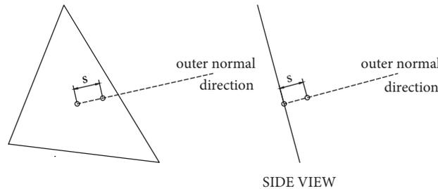
**Figure 8.** The change of position of the singular point on a triangular element.
