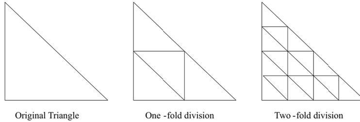
**Figure 2.** Subdivision by folding as presented in [29] using Romberg integration scheme.
