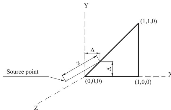
**Figure 6.** The location of the source point and the integrated triangular element for the benchmark problem. The triangle is a right-angled triangle at xy-plane and the source point is located at  $(\Delta, \Delta, z)$ .
