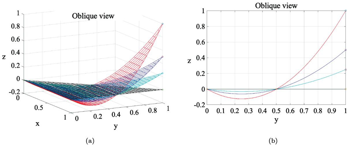
**Figure 7.** The curvature of the isoparametric quadratic six-noded element. The tip z-coordinate values are:  $M = 1$  (red),  $M = 0.5$  (blue),  $M = 0.25$  (green) and  $M = 0$  (black). Note that for  $M = 1$  the element is planar and identical to three-noded linear isoparametric element.
