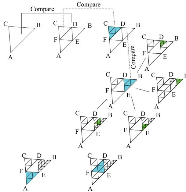
**Figure 5.** The subdivision of the integration region into similar triangles. Each subdivision level is represented with a different color. The self-localization behavior of the algorithm can be traced in the triangle region  $BE D$ .
