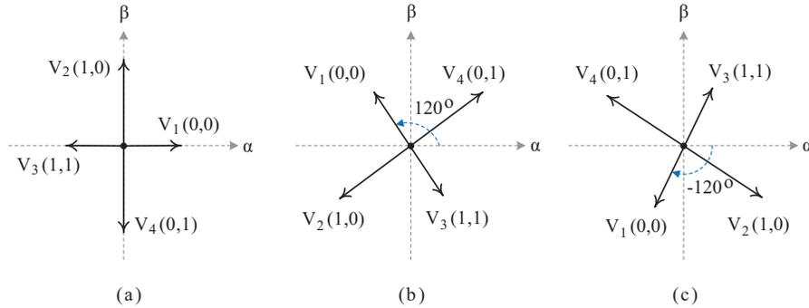
**Figure 4.** Space vector diagram of FSTPI (a) connection of phase-A to the center tap, (b) connection of phase-B to the center tap, (c) connection of phase-C to the center tap.
