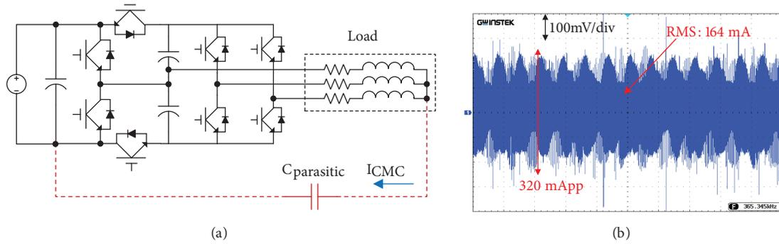
**Figure 12.** Common-mode current (a) circuit model for test, (b) common-mode current waveform.
