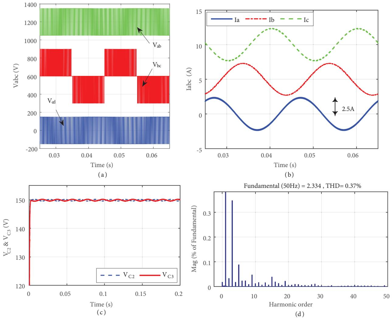
**Figure 7.** Waveforms of the SCFSTPI (a) output voltages, (b) output currents, (c) capacitors voltages, (d) output current THD.
