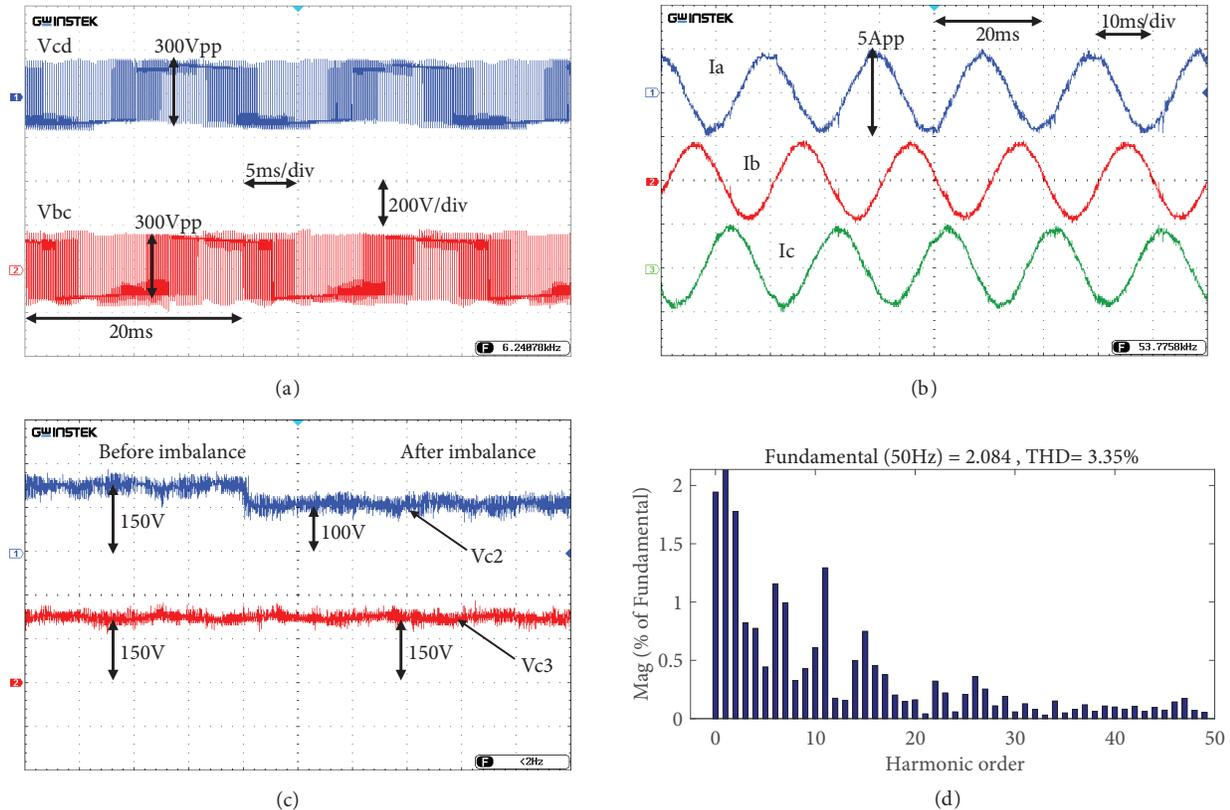
**Figure 11.** Key waveforms of the SCFSTPI under the voltage imbalance problem (a) output voltages, (b) output currents, (c) capacitors voltage, (d) current THD.
