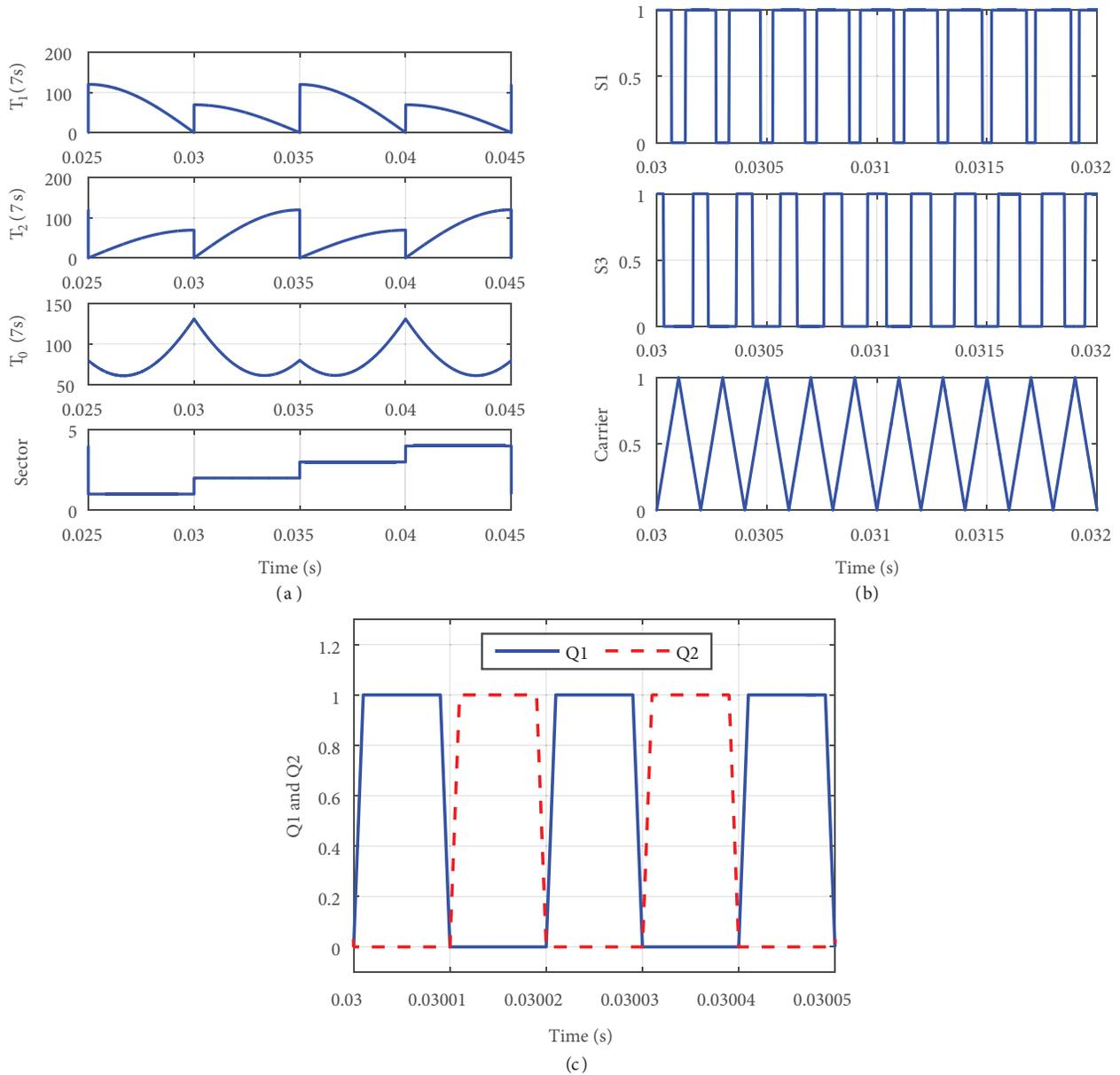
**Figure 6.** Waveforms of the control system (a) dwell-times for one cycle of output voltage respect to sector change, (b) command signals of S1 and S3 subject to the carrier waveform, (c) command signals for SC stage.
