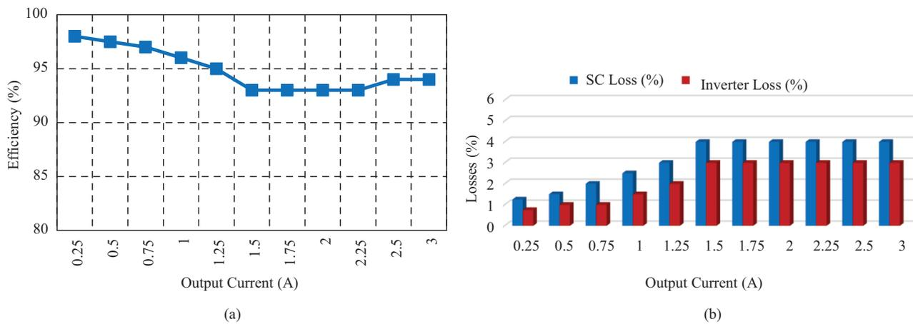
**Figure 13.** Efficiency analysis (a) overall efficiency curve vs. output current in experiments, (b) each stage losses vs. output current.
