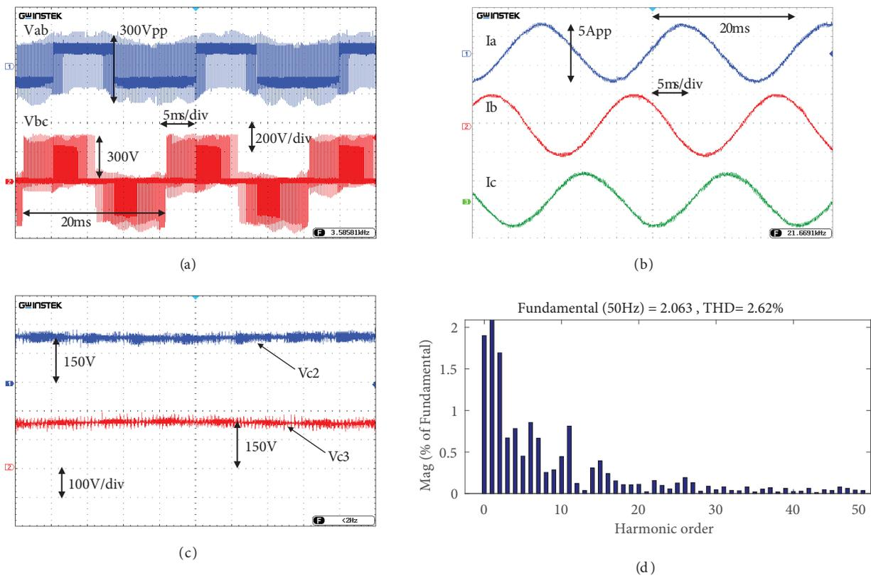
Figure 10. Waveforms of the SCFSTPI under normal condition (a) output voltages, (b) output currents, (c) capacitors voltage, (d) current THD.
