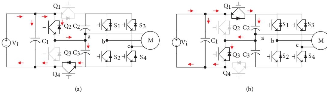
**Figure 2.** Switching states of SC circuit, (a)  $Q_1$  and  $Q_3$  are on, (b)  $Q_2$  and  $Q_4$  are on.
