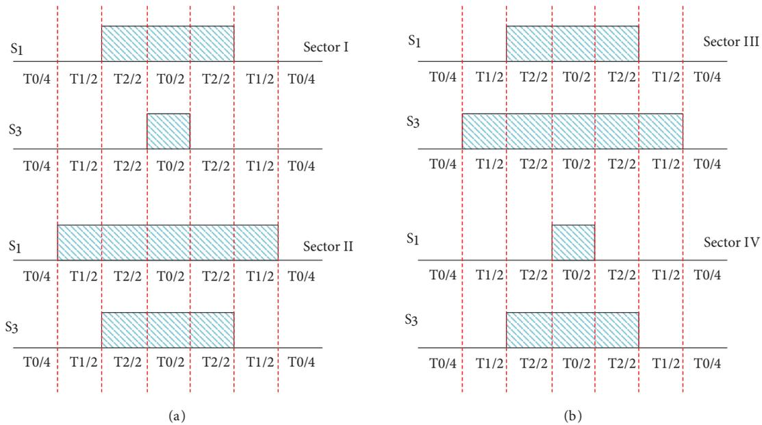
**Figure 5.** Switching sequences of the proposed FSTPI-SVM (a) switching strategy of Sectors 1 and 2, (b) switching strategy of Sector 3 and 4.
