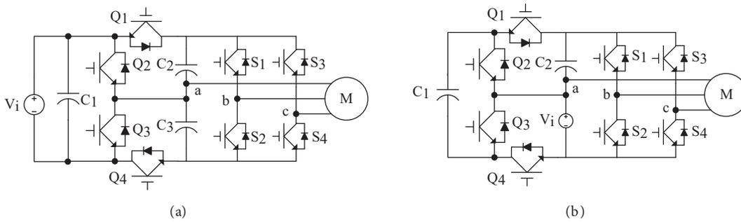
**Figure 1.** Circuit schematic of the proposed converter (a) first configuration, (b) second configuration.
