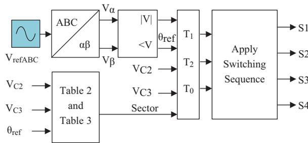
**Figure 3.** Control diagram of the proposed SCFSTPI.
