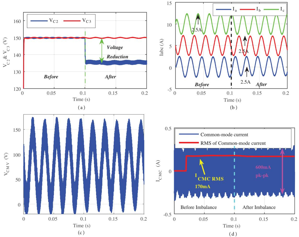
**Figure 8.** Key waveforms of the SCFSTPI under voltage imbalance condition (a) capacitors voltages, (b) output currents, (c) common-mode voltage, (d) common-mode current (RMS value = 170 mA).
